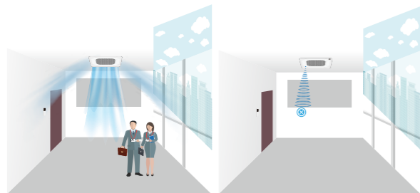
The indoor unit automatically runs when detecting human body
