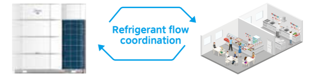
Automatic calculation of building load and required refrigerant volume based on sensor parameters.
